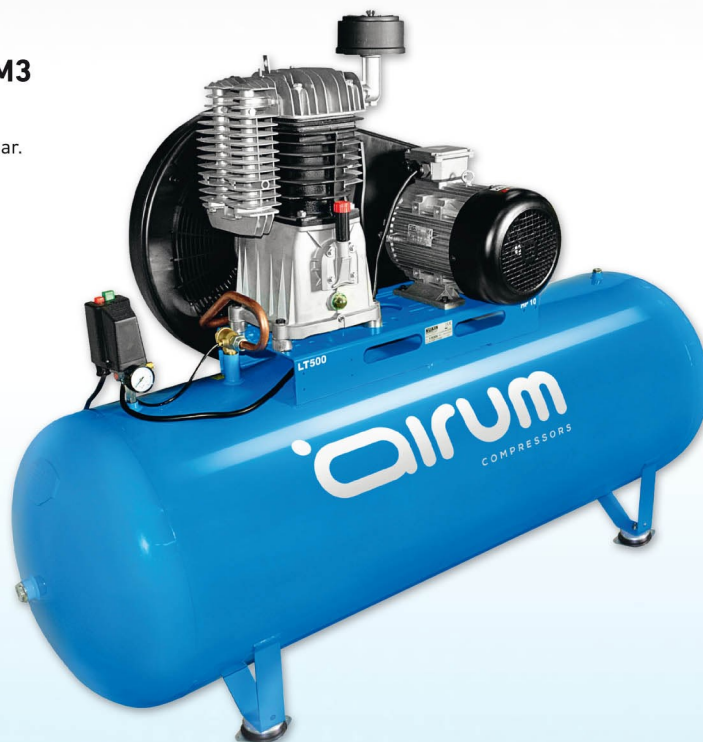
NB4/270 FT 5.5 Airum 5.5 hp caldera 270 lts. 550 lts./min. 400V III 11 bar.
